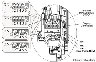
Fig. 9 — Outdoor Sensor Connection
